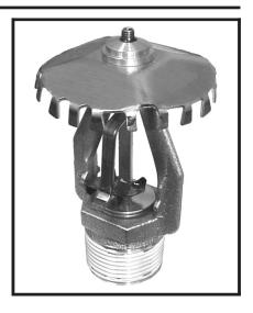
Discharge Coefficient K = 25.2 GPM/psi<sup>1/2</sup> (362,9 LPM/bar<sup>1/2</sup>)
